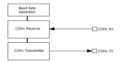
A single-byte serial transmission consists of the start bit, 8 bits of data followed by the stop bit. The start bit is always 0, while a stop bit is always 1. The LSB (Least Significant Bit, Bit 0) is sent out first following the start bit.
