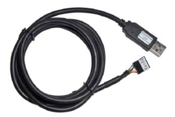
A 4D Programming Cable can connect directly to the gen4 Interface board (gen4-IB), which ship with each gen4 Display Module (unless otherwise stated). Simply connect the supplied 30-way FPC cable into the ZIF connector on the gen4 Interface Board, and connect the Programming Cable into the 5-way header on the Interface Board.
