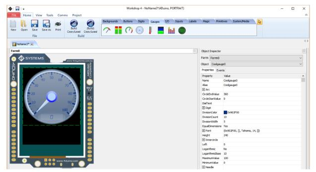
Each object has parameters that can be set, such as colour, range, text, etc. It is then just a case of selecting the event the object is to be associated with — such as sending the value to the Atmel or directly interfacing to another object, it is that simple. In seconds you can transform a blank display into a fully animated GUI with moving sliders, animated press and release buttons, and much more.
