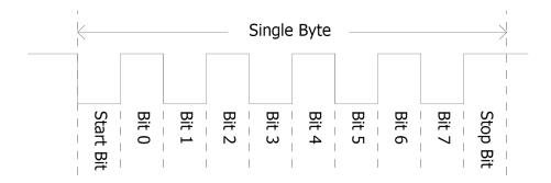
uLCD-70D Series Serial Ports - TTL Level
