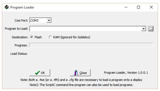
**Program Loader** is a GUI interface designed to download Applications to either Flash or RAM, useful for testing or production loading, without the need for Workshop4 itself.
