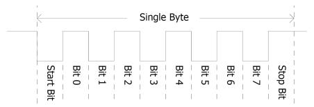
gen4-uLCD-(43-70)D Series Serial Ports - TTL Level
