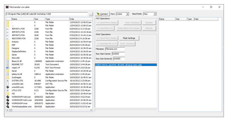
File Transfer can be used for loading SPI Serial Flash Memory or the micro-SD card. When actioning the programming process from Workshop4, the appropriate one will be loaded based on your hardware and software settings.
