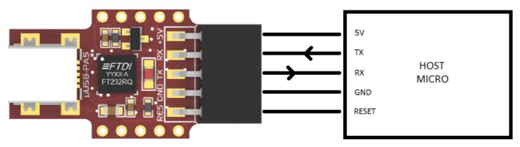
The micro USB is designed to have a compact footprint, and be compatible with prototyping such as plugging it directly into a breadboard when male 2.54mm (0.1") headers are soldered to the row of 5 pins, along each side.
