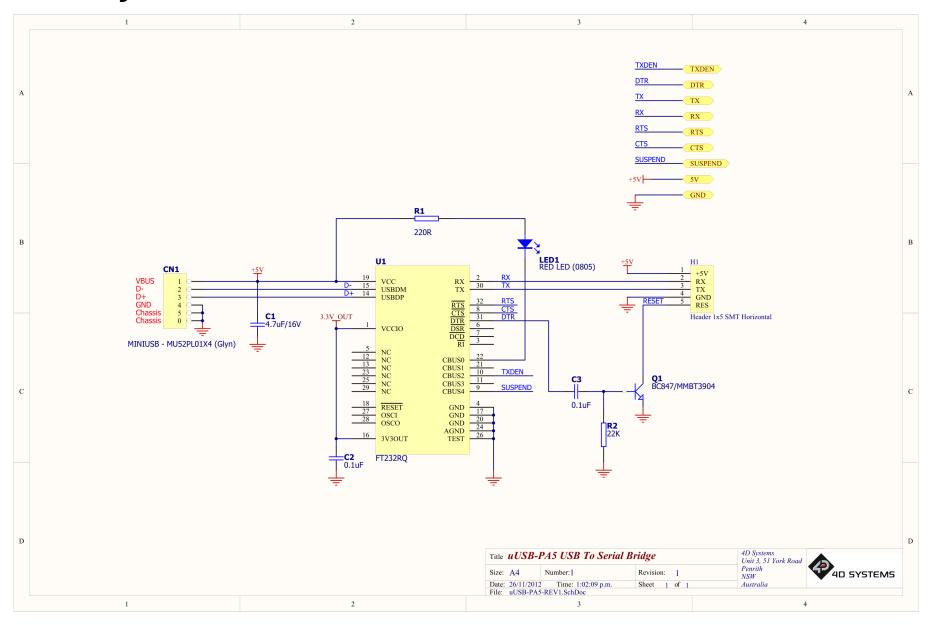
uUSB-PA5 Schematic Diagram HW REV 3.0
