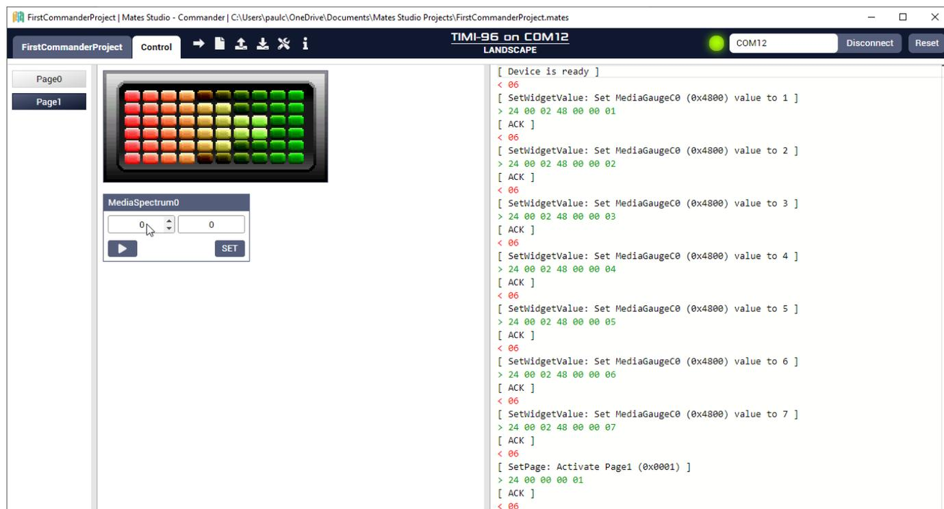
All spectrums, regardless of the amount of bars will only have a single widget input control but contain a 2nd value to set the required bar with a value.
