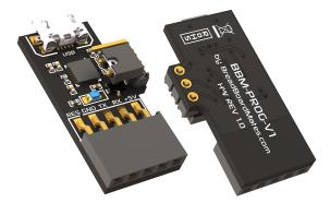
The BBM-PROG features a 3-pin jumper with a shunt, which is present to change the way the programmer handles the Reset line, used by TIMI and other devices.
