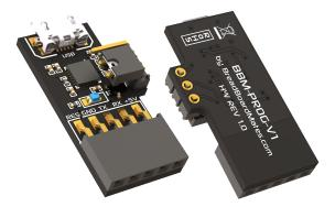
The BBM-PROG features a 3-pin jumper with shunt, which is present to change the way the programmer handles the Reset line, utilised by TED-96 and other devices.
