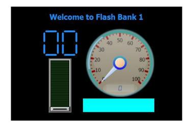
This is because the processor runs the program from flash bank 0 always after a power cycle.
