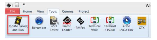
With the display module connected to the PC thru a programming module, click on the Upload Bank(s) and Run icon. This program needs to be loaded to flash bank 0 of the display module only once. After the Upload Bank(s) and Run program is loaded flash bank 0, the display module now shows the message indicated below.
