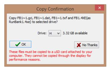
As indicated in the image, WS4 will copy four files to the uSD card. FB1~1.4XE is the actual program file. This will be copied to the uSD card as "RunBank1.4XE". The other files are supporting graphics and font files.
