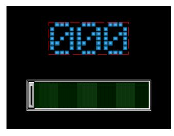
The projects developed in this application note demonstrate CustomDigits linked to the changes of a Slider widget. The user moves or touches the Slider, and the CustomDigits change their values to correspond with the Slider's change in value.
