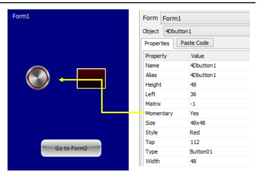
The object 4Dbutton1 is used for Form1 to have another touch objects besides Winbutton1. This also turns the ON the Userled1.
