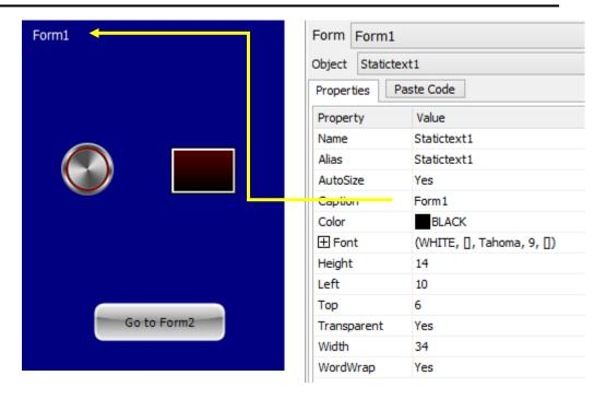
The object Statictext1 is used to indicate that the current form is Form1.
