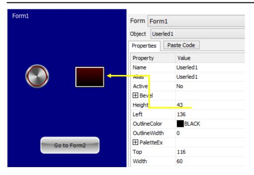
The object Userled1 is used an output for the 4Dbutton1. If 4Dbutton is pressed, Userled1 will turn ON, else it will turn OFF.
