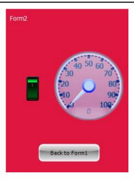
Form2 contains a background color of CRIMSON, 4Dbutton, Cool Gauge, Winbutton and a Statictext. If 4Dbutton2 is pressed the Coolgauge1 will start to move from 1 to 100, else if 4Dbutton2 is not pressed then Coolgauge1 will stay at 0 value. Winbutton2 object is used to go back to Form1. Statictext2 is used to indicate that the current form is Form2.
