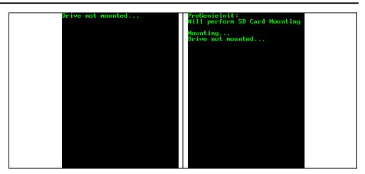
As seen in the image above, the display prints first the "PreGenie:Init: Will perform SD Card Mounting" and then after 3000 ms, the display will print "Mounting... Drive not mounted...". If an SD card is still not inserted in the display then it will continue to print "Drive not mounted..."
