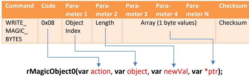
**Diagram A. Implementation of the General Model Using a Magic Object**
