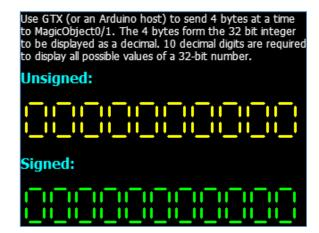
Use GTX (or an Arduino host) to send 4 bytes at a time to MagicObject0/1. The 4 bytes form the 32 bit integer to be displayed as a decimal. 10 decimal digits are required to display all possible values of a 32-bit number.
