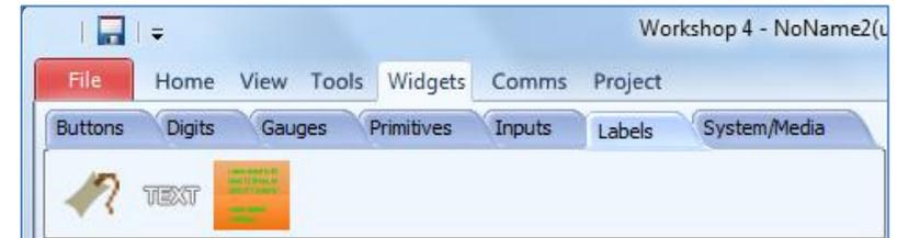
Click inside the display area in the Form or WYSIWYG section of WS4 IDE to drop the **String** placeholder represented by a dashed red box.
