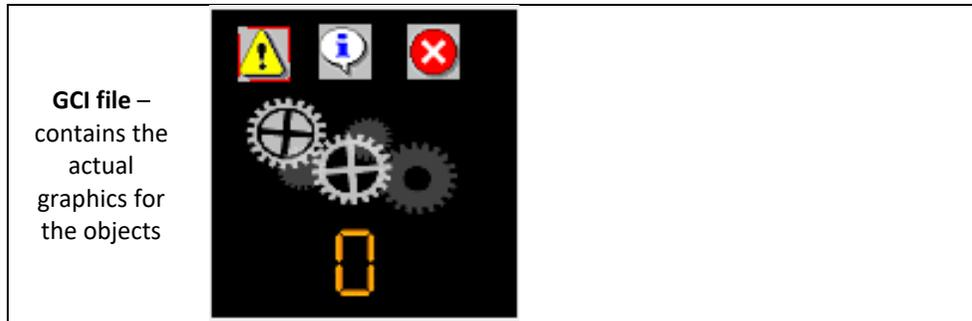
When the user intends to display a hundred images for instance, the Graphics Composer is first used to combine them into a GCI file and to create a DAT file. The user will then write a program to access these two files to be able to display the images on the screen. Below is a screenshot of the Graphics Composer, the use of which is discussed in the following section.
