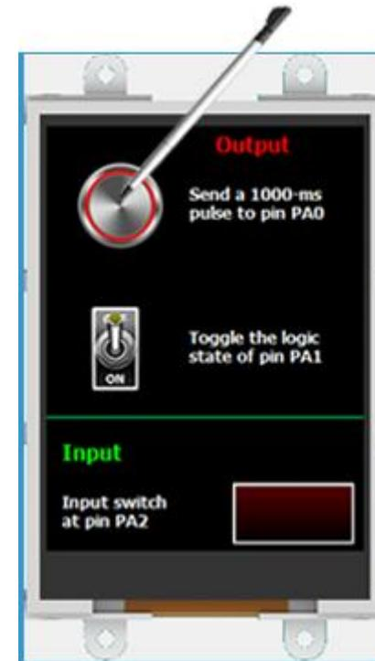
Upon releasing 4Dbutton0, the green LED should light up for one second (approximate). Also, a message is sent from the display module to the PC. The message is displayed on the white area on the right part of the GTX Tool window.
