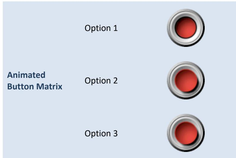
The animated button automatically plays a sequence of images when it is pressed and released. The user provides the image to be used for each state and defines the frame delay. The figure to the left shows an animated button with five states or frames.
