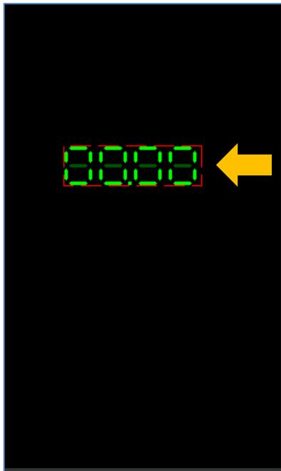
The object can be dragged to any desired location and resized to the desired dimensions. The **Object Inspector** on the right part of the screen displays all the properties of the newly created LED digits object named **Leddigits0**.
