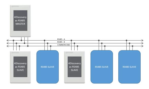
Typical 2-wire RS485 configuration, which includes a common ground
