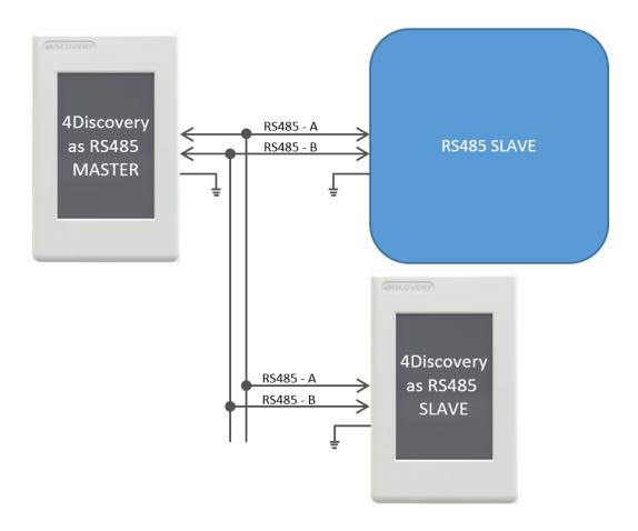
4Discovery as the Master of the RS485 Bus with multiple Slaves, which can include multiple 4Discoverys (as Slaves).
