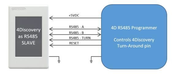
Programming the 4Discovery using the 4D RS485 Programmer
