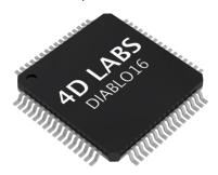
The DIABLO16 is a smart Controller and the interface to the TFT- LCDs is almost plug-n-play. All of the data and control signals are provided by the chip to interface directly with the display.
