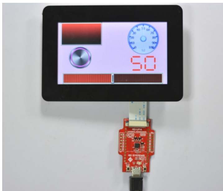
Typical connection of gen4 display module (gen4-uLCD-43DCT-CLB) to 4D-UPA
