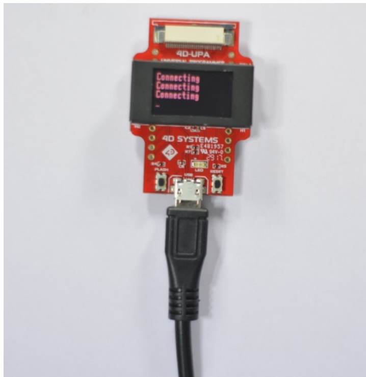
Connection of an IoD-09TH Display module to 4D-UPA with a micro-USB Cable
