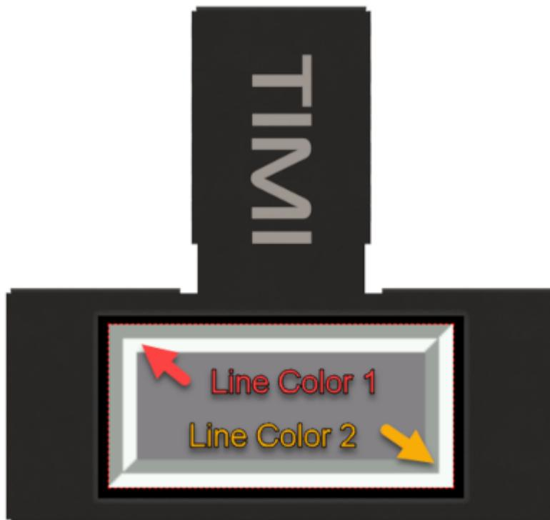
If the Panel State property is set to Raised then Line Colour 1 and Line Colour 2 are as shown below.
